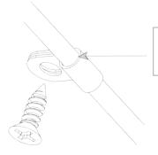
The wire must be in the «O» so that it is not crushed.
